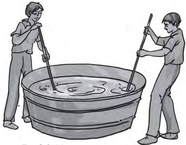
Fig. 3.8 (b) Scouring in tanks
