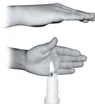
Fig. 4.10 Transfer of heat by convection in air
