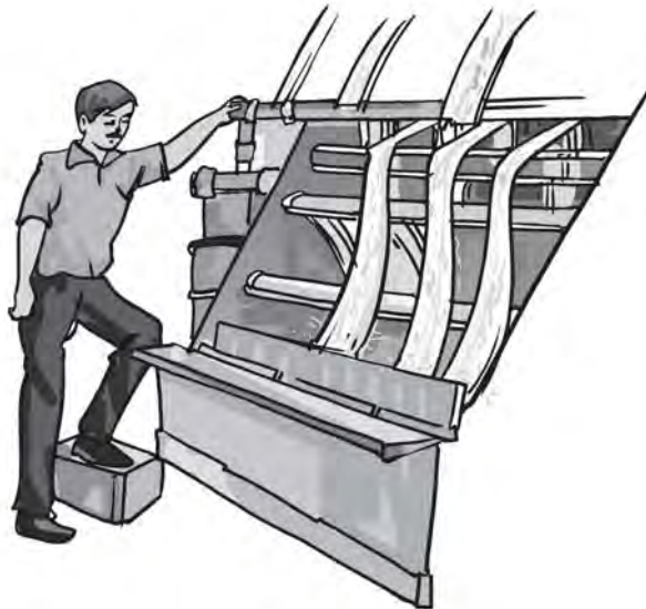
Fig. 3.8 (c) Scouring by machines
