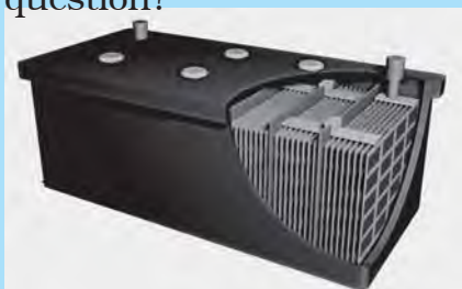
Fig. 14.6 Truck battery and its cutout
