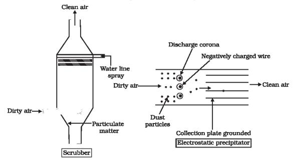
Figure 16.1 Electrostatic precipitator
