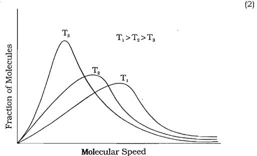
When temperature is decreased; the height of the peak increases. Hence, the fraction of molecules having lower speeds (lower energy) increases. (1)
