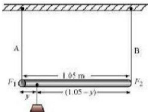
Taking torque about the point of suspension, we have:  $F_1 y = F_2 (1.05 - y)$
