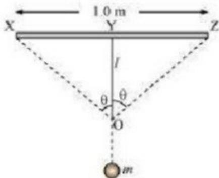
Original length = XZ Depression = l The length after mass m, is attached to the wire = XO + OZ Increase in the length of the wire: Original length = XZ Depression = l The length after mass m, is attached to the wire = XO + OZ Increase in the length of the wire:
