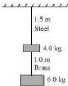
**Ans :** Elongation of the steel wire =  $1.49 \times 10^{-4}$  m Elongation of the brass wire =  $1.3 \times 10^{-4}$  m Diameter of the wires,  $d = 0.25$  m Elongation of the steel wire =  $1.49 \times 10^{-4}$  m Elongation of the brass wire =  $1.3 \times 10^{-4}$  m Diameter of the wires,  $d = 0.25$  m
