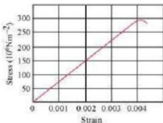
**Ans :** (a) It is clear from the given graph that for stress  $150 \times 10^6 \text{ N/m}^2$ , strain is 0.002  $\therefore$  Young's modulus,  $Y = \frac{150 \times 10^6}{0.002} = 7.5 \times 10^{10} \text{ N/m}^2$  (a) It is clear from the given graph that for stress  $150 \times 10^6 \text{ N/m}^2$ , strain
