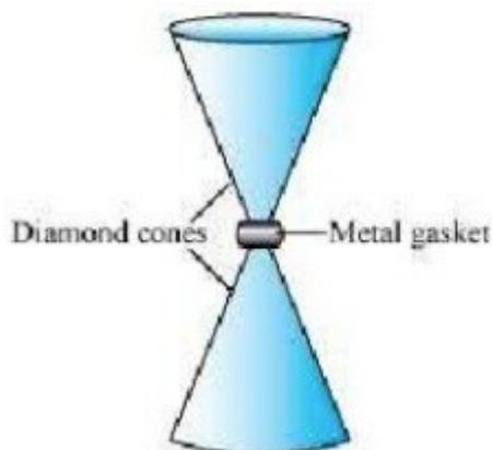
**Ans :** Diameter of the cones at the narrow ends,  $d = 0.50 \text{ mm} = 0.5 \times 10^{-3} \text{ m}$  Radius,  $r = d/2 = 0.25 \times 10^{-3} \text{ m}$  Compression force,  $F = 50000 \text{ N}$  Pressure at the tip of the anvil: Diameter of the cones at the narrow ends,  $d = 0.50 \text{ mm} = 0.5 \times 10^{-3} \text{ m}$  Radius,  $r = d/2 = 0.25 \times 10^{-3} \text{ m}$  Compression force,  $F = 50000 \text{ N}$  Pressure at the tip of the anvil:
