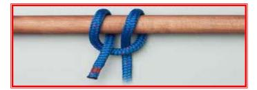
(d) **<u>Rollinghitch</u>**. This hitch also used for securing a rope to a spar, rail or similar fitting when the pull is expected to be from one side or the other
