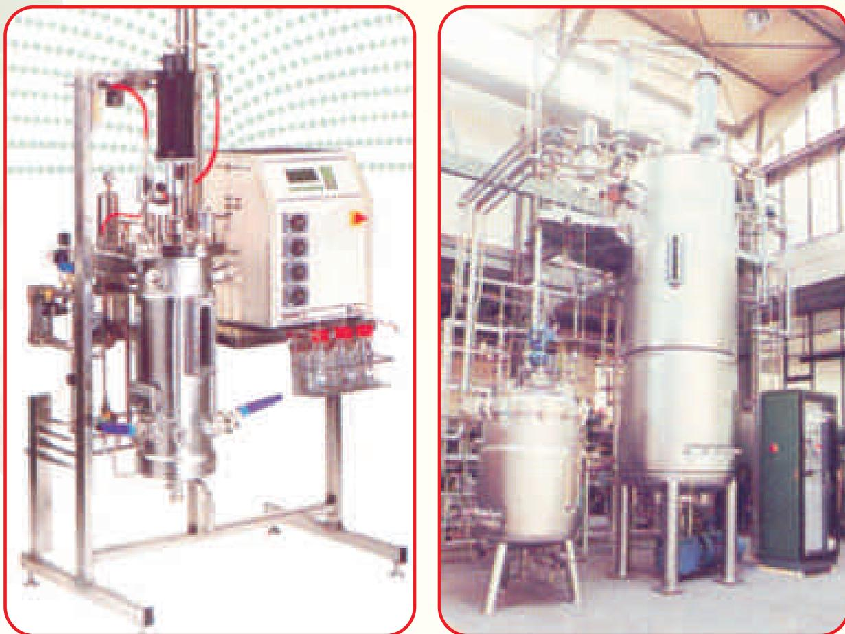
Fig. 4. (A) Laboratory-scale fermentor; (B) Industrial-scale fermentor.
