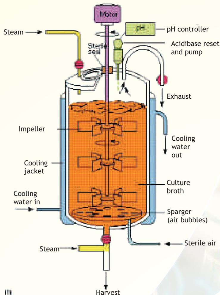
**Fig. 3.** Basic features of a fermenter (Bioreactor).
