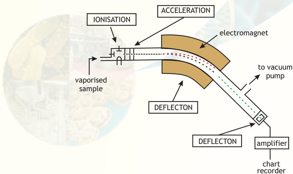
**Fig. 10.** An outline of a mass spectrometer.
