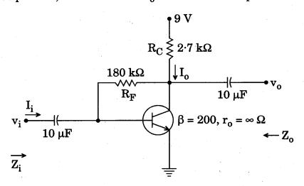
(ii) Draw the equivalent circuit (hybrid- $\pi$  high frequency model) of the CB amplifier shown below. Find an expression for the high-frequency voltage-gain ratio. Also describe the high-frequency behaviour of this amplifier.
