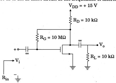
The effect of channel length modulation on the dc operating point can be neglected.
