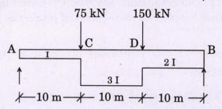
Using conjugate beam method, for the beam shown below, find the slopes and deflections at 'A', 'B', 'C' and 'D'. Given :  $E = 200 \times 10^6 \text{ kN/m}^2$  and  $I = 300 \times 10^{-4} \text{ m}^4$ . Neglect the weight of the beam.
