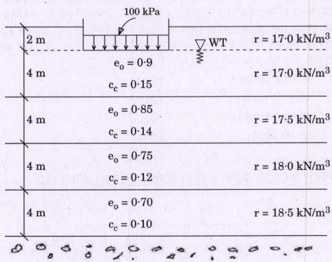
A 15 m long and 10 m wide raft is placed on a 16 m thick clay deposit, consisting of 4 sub-layers as shown in the figure below. Determine the settlement of the raft foundation because of the consolidation of the clay layers. Assume unit weight of water,  $\gamma_{\rm w} = 9.81~{\rm kN/m^3}$ .
