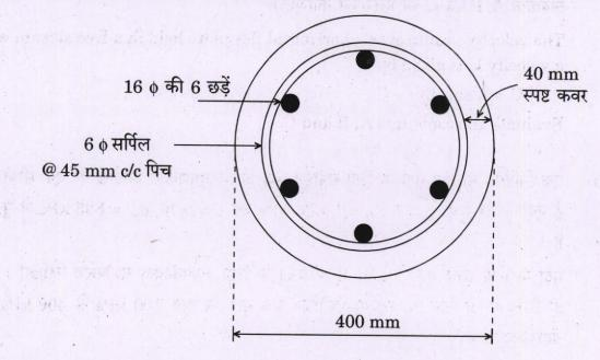
A column has an unsupported length of 3.4 m and is effectively held in position at its both ends, but not restrained against rotation. The cross-section of the column and reinforcement details are shown in the figure below. Determine the safe axial load that the column can carry. Use M 25 grade of concrete and Fe 415 grade of steel.
