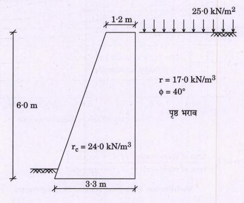
The earth retaining wall shown in the figure is to support a backfill of granular soil, which has unit weight of  $17.0 \text{ kN/m}^3$  and angle of internal friction of  $40^\circ$ . The wall also supports a surcharge of  $25.0 \text{ kN/m}^2$  as shown in the figure. The coefficient of base friction is 0.5. Determine the factor of safety against sliding and overturning for the wall. Also determine the maximum and minimum vertical pressure below the base of the retaining wall.
