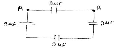
Find out equivalent capacitance between the points A and B in the following circuit :
