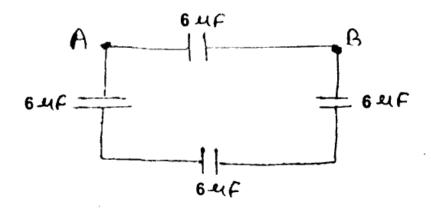
Find out equivalent capacitance between the points A and B in the following circuit :
