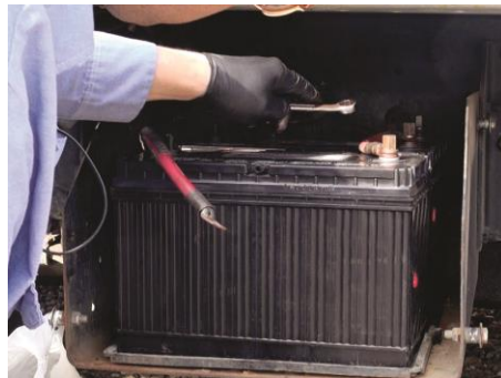
Fig.1.10 DC voltage source in truck, Courtesy: http://bit.ly/2MfJgSh
