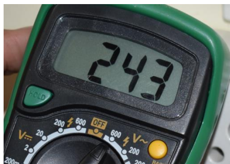
Fig.2.9 Holding the value in the display using hold button
