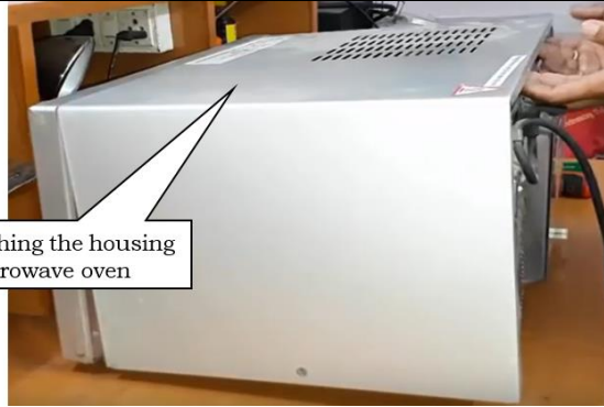
Fig.4.5 Slide to remove the housing
