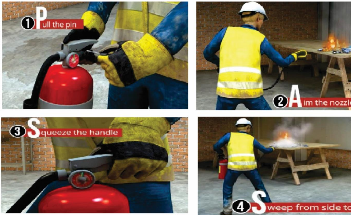
Fig.5.28 Steps to open the seal and safety pin
