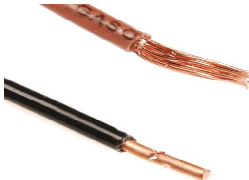
Fig.5.14 Damage on the conductor
