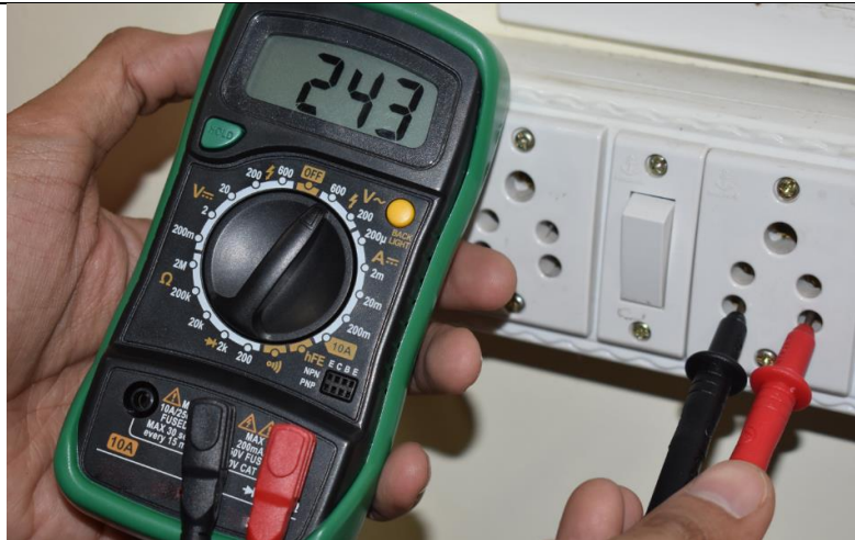
Fig.2.7 Measuring AC voltage using multimeter
