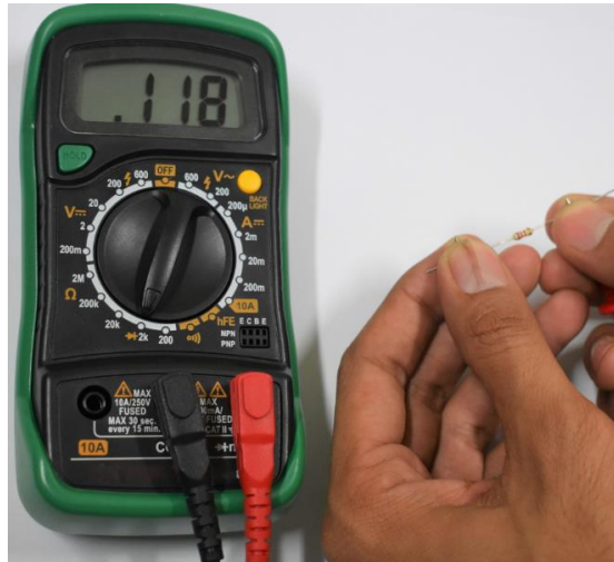
Fig.2.3 Measuring the resistance of resistor by touching the resistor terminal to the red and black probes
