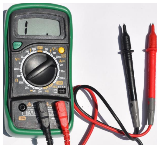
Fig.2.2 Multimeter knob switched to measure the resistance value
