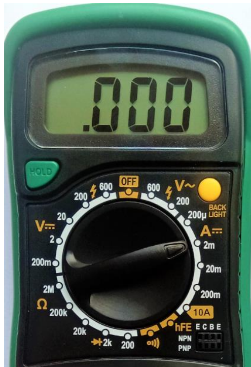
Fig.2.15 Hold button can be used to stabilised the value
