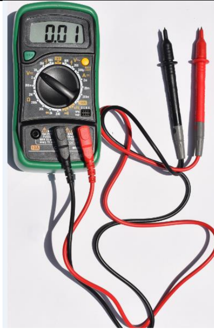
Fig.2.5 Connecting the red probe to the volt terminal and black probe to the common terminal
