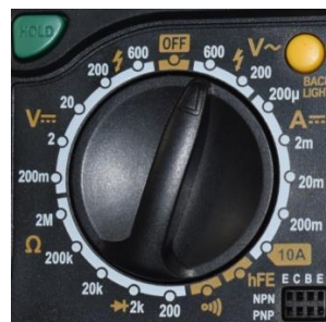
Fig.2.6(b) Turning the knob to measure the AC voltage
