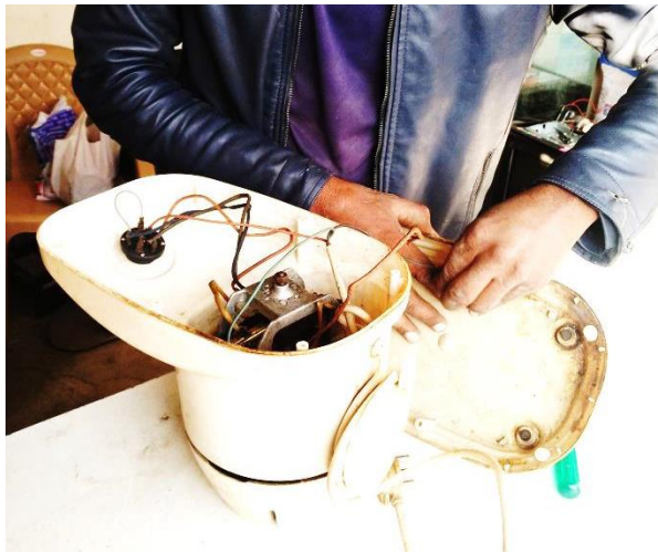
Fig. 3.69 Unlocking the housing of motor
