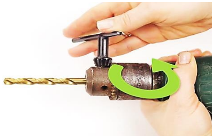
Fig.2.25 Turn the key in counter clockwise direction
