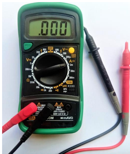
Fig.2.11 Set the multimeter to measure the current
