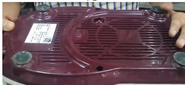
Fig. 3.20: Overload protection button in a mixer/grinder
