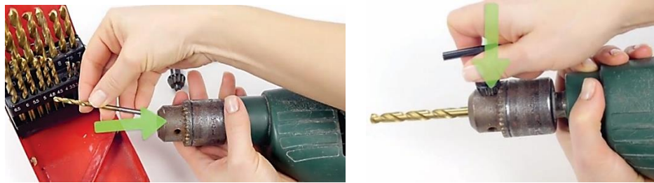
Fig.2.27(a) Insert the bit and tighten it, Fig.2.27 (b) By rotating the key in clockwise direction, Courtesy: http://bit.ly/2KBznwG
