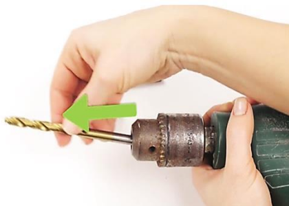
Fig.2.26 Pull the bit to remove out from the chuck
