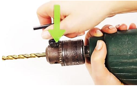
Fig.2.24 Inserting the key in order to loosen the chuck, Courtesy: http://bit.ly/2KBznwG
