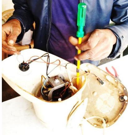
Fig. 3.68: Reassembling of motor
