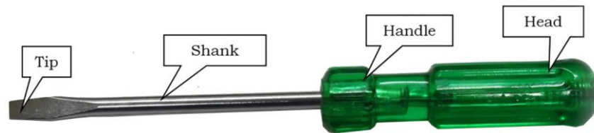
Fig.2.19 Parts of screwdriver
