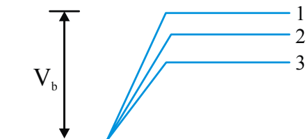
Fig. p-n junction diode under forward bias. Barrier potential (1) without battery, (2) low battery voltage, and (3) high voltage battery.
