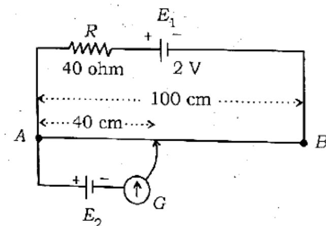
In null deflection position of the galvanometer (G), calculate the e.m.f. of the cell  $E_2$ .
